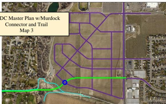
The proposed USDC Master Plan w/Murdock Connector and Trail follows the master plan with the addition of the roundabout, which will align traffic across the pipeline.
